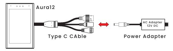
Mode 1: Connect directly to the power adapter
