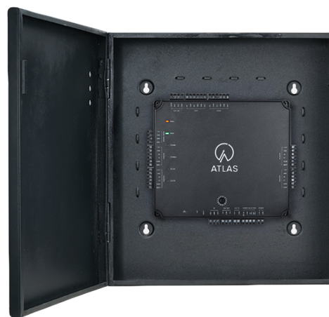
Includes panel, power supply & metal enclosure
